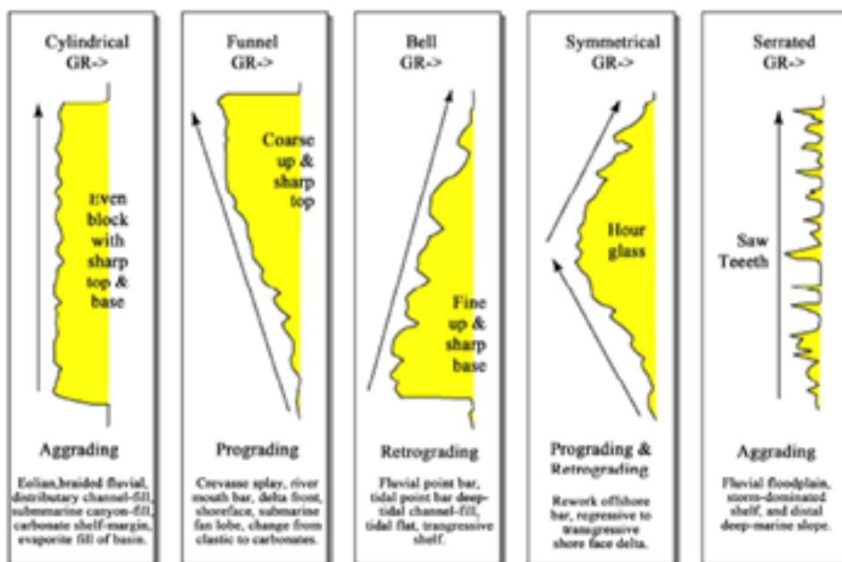
Fig. 2: Well log response character for different environments (Onyekuru et al. 2012).
